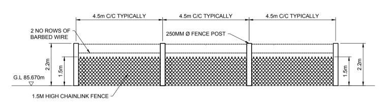
SITE PERIMETER FENCE DETAIL SCALE 1:100
